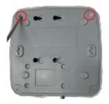
① Loosen the screws on the bottom of the chassis.
