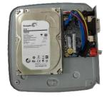
② Align the HDD with the four holes in the bottom.
