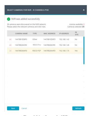
Figure 8 Select Camera for NVR
